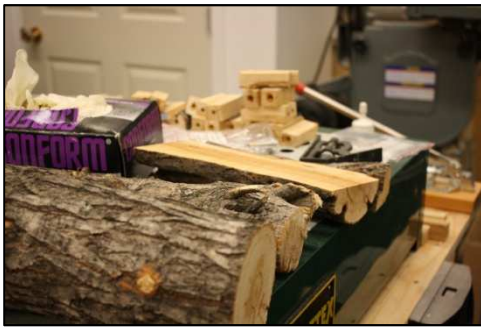
Diamond willow pieces are formed into blocks, then drilled through the middle for the
