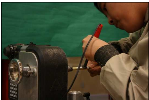
Diamond willow pieces are formed into blocks, then drilled through the middle for the
