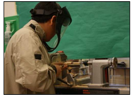
Trey Timbre uses a lathe to shape his blocks of wood to the shape of a pen
