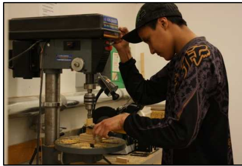
Brent Kotchea prepares a block for the lathe using a drill press.
